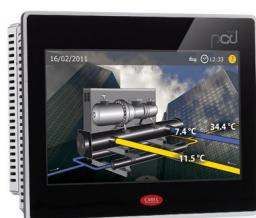
Number of smart features can be optionally installed to connect the unit to BMS (building management system), control it from the WEB, or make human control more user friendly.
