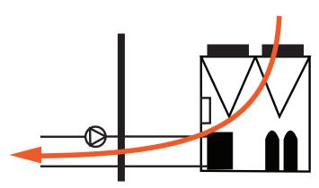
Heat transfer from cold ambient air to hot fluid.
