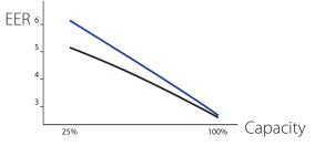
Inverter compressors chiller EER in part load.
