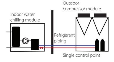
In the most of northern Europe regions the brine is required for outdoor installation. But you can chill water directly if buy remote evaporator units from us. You need to install refrigerant piping between two modules supplied from us - outdoor and indoor. Like in residential air conditioner. And the indoor module will chill the water directly.
